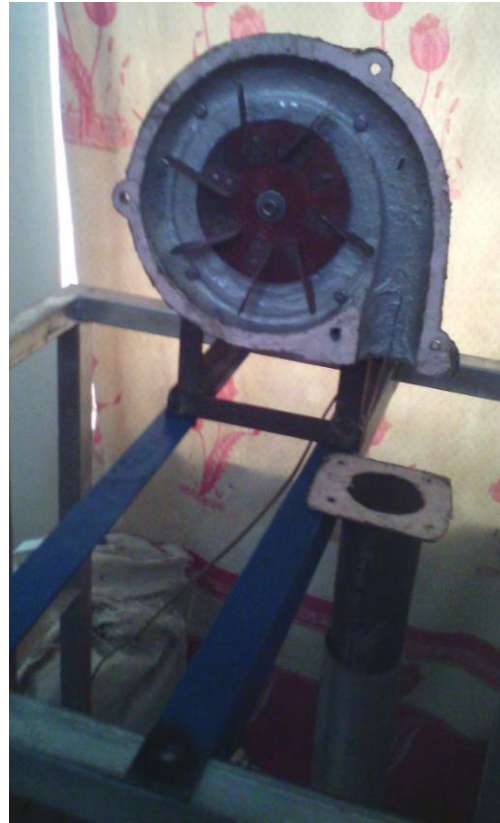
(b) Mounted air blower
